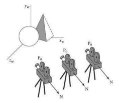
✓ Alternatively, different views of an object or group of objects can be generated using geometric transformations without changing the viewing parameters
