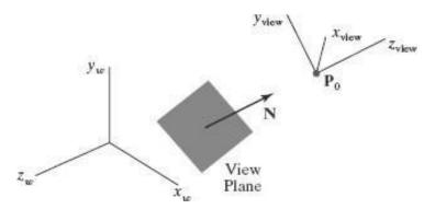
✓ An additional scalar parameter is used to set the position of the view plane at some coordinate value  $z_{vp}$  along the  $z_{view}$  axis,
