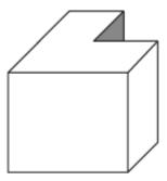
✓ In general, back-face removal can be expected to eliminate about half of the polygon surfaces in a scene from further visibility tests.
