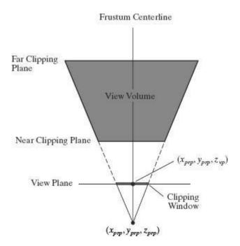
✓ Because the frustum centerline intersects the view plane at the coordinate location ( $x_{prp}$ ,  $y_{prp}$ ,  $z_{vp}$ ), we can express the corner positions for the clipping window in terms of the window dimensions:
