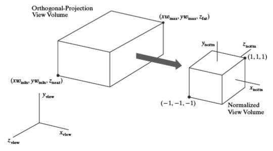
• The normalization transformation for the orthogonal view volume is
