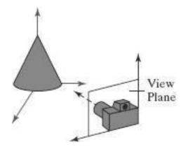
Coordinate reference for obtaining a selected view of a three-dimensional scene.
