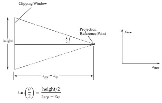
✓ so that the clipping-window height can be calculated as
