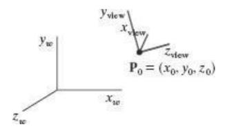
A right-handed viewing-coordinate system, with axes  $x_{view}$ ,  $y_{view}$ , and  $z_{view}$ , relative to a right-handed world-coordinate frame.
