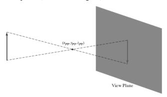
✓ Perspective effects also depend on the distance between the projection reference point and the view plane, as illustrated in Figure below.
