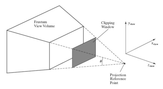
✓ For a given projection reference point and view-plane position, the field-of view angle determines the height of the clipping window from the right triangles in the diagram of Figure below, we see that
